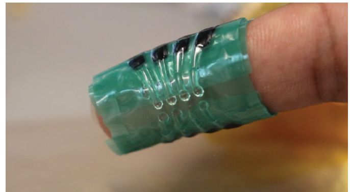
Fig. 1. The high-resolution ElectroHydraulic Haptic Interface worn over fingertip. It consists of 16 individually controlled miniaturized electrohydraulic bubble actuators capable of rendering high intensity fine-tactile pressure (up to 34 kPa) as well as wide bandwidth vibrotactile feedback (up to 700 Hz) within 1 cm 2 .
